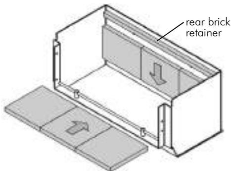
The side firebricks have an angled cut on the top edge. Place these firebricks into the firebox so that the shorter edge is at the rear of the firebox and the longer edge is at the front.
