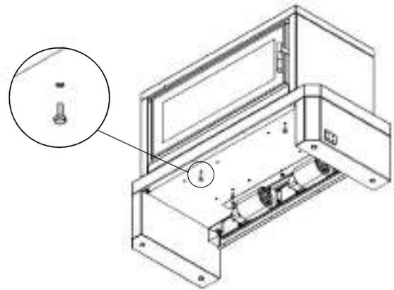
Replace the cover panel and fix into place with the 8 screws.
