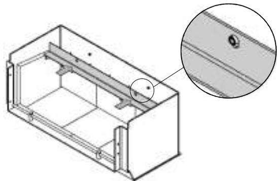
Place the front baffle holder into the firebox. This sits on top of the side firebricks towards the front of the firebox. There are two locating holes in the holder that sit over pins at the front of the firebox.
