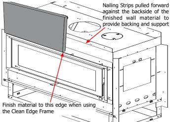
5. Install the steel framing: Both walls require construction of non-combustible materials including the framing. Steel stud framing must be used. Install the left and right vertical steel frame and secure to the nailing strips. Position the steel frame behind the nailing strip. Install the top horizontal steel frame and secure to the top nailing strip.
