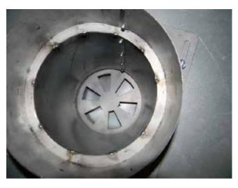
View with Cover Plate removed and unit adapter installed - primary air control now visible.
