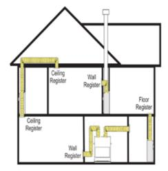
Diagram 1: Guide for possible air duct runs and locations. Keep duct length and number of bends to a minimum. **Maximum duct length is 9.0m.** The Fan Kit 946-591 does not contain any flexible duct. A separate Flex Kit is required 946-596. This Flex Kit contains one length of 4.5 metres of flex duct. If 9.0 metres of flex ducting is required you will need to purchase an additional Flex Kit.
