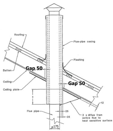
Typical Example of a Sloped Ceiling Penetration
