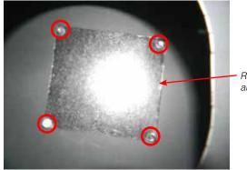
Remove screws and Cover Plate
