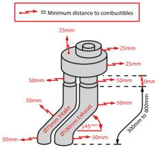
\*Note: Underside of converter box can be fixed straight onto wooden joists. \*\*Note: Flexi-Flue must not be run at an angle greater than 45 degrees from vertical; excluding all appliance built into a freestander kit.
