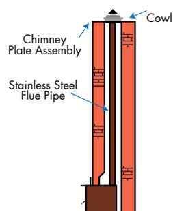
**FLUE KITS** Coonara heaters are designed and tested for use with Coonara approved Flue kits to Australian Standard AS2918 to enable the specified clearances to combustible materials.
